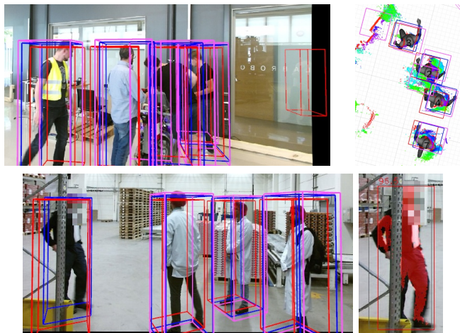
Fig. 3: Detections of our YOLO v3-based method in blue, Mobility Aids in magenta, RGB-D Pose 3D in red. Upper row shows false alarms of [7], [17], lower row a false depth estimate of [17], which we avoid via instance segmentation.
