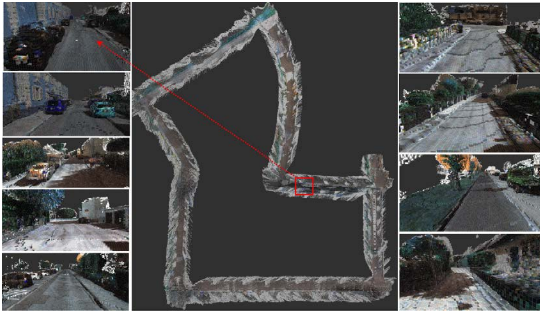
Fig. 7: The center image is the global dense 3D map of sequence 07 in the KITTI dataset. The small images in the surrounding show enlarged local areas of the global map.
