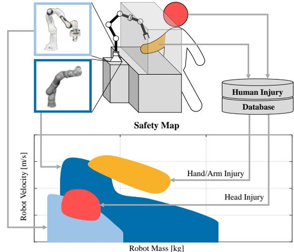
Fig. 1. *Safety map* concept. The global or task-specific (gray interaction area) mass/velocity ranges of different robots (here: DLR Lightweight Robot and Franka Emika Panda) and injury occurrence of human body parts are represented in a unified manner in the *safety map*. The injury data associated with the considered body parts is obtained from an injury database.
