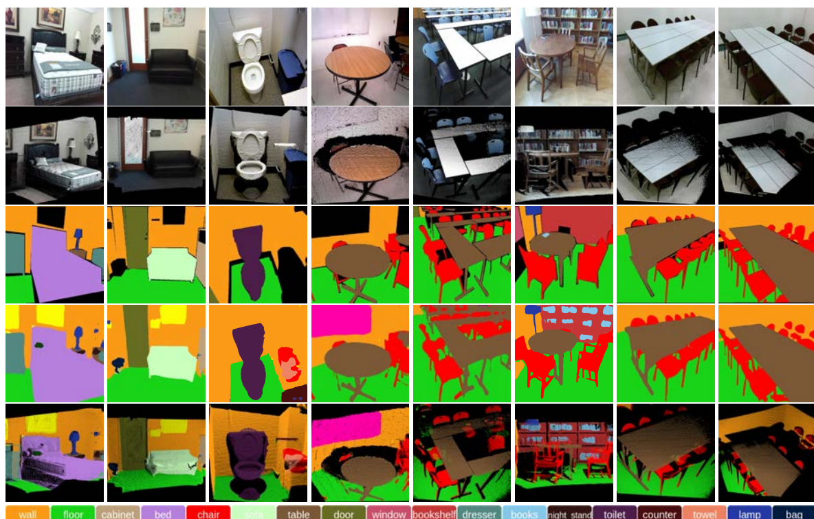
Figure 6. Qualitative results (best viewed in colour) for the Pixel-Voxel network on the SUN RGB-D dataset. For different scenes in each row, the following images are displayed: RGB image (Row 1), 3D point cloud (Row 2), ground truth image (Row 3), 2D semantic image (Row 4) and 3D semantic point cloud (Row 5). The Pixel-Voxel network produces results with accurate boundary shape such as the shape of the bed, toilet and especially the legs of the furniture.
