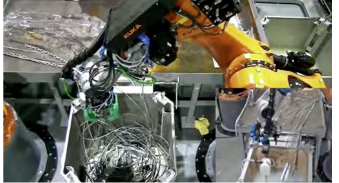
Fig. 1. In this figure, a robot is sorting nuclear waste (metal strings and chains) into a segregation bin through teleoperation.
