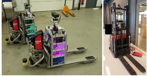
Figure 2: Two types of autonomous guided vehicles which were used to record the real-world RGB-D intralogistics dataset (with a Kinect v2) for validation and testing.
