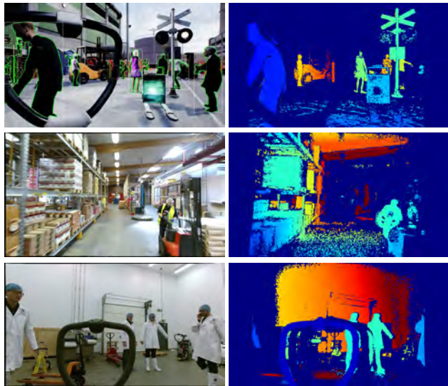
Figure 1: Using Unreal Engine 4, we synthetically generate crowded RGB-D sequences to train robust person detectors. We evaluate performance of the resulting YOLOv3 models on a challenging intralogistics dataset which we recorded. In the top image, red contours denote small groundtruth objects that we filtered out during training for better results.
