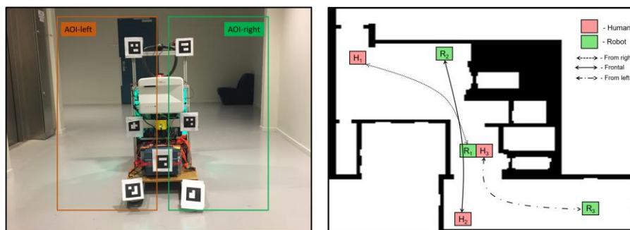
Figure 1. (Left) Robot platform used for the experiments and the pre-defined Areas of Interest (AOI): AOI-left (Orange) and AOI-right (Blue). (Right) Experimental layout design: During the experiment, the humans (denoted by H_i ) moved from H_i \rightarrow R_i and the small forklift robot (denoted by R_i ) moved from R_i \rightarrow H_i .
