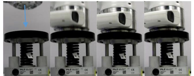
Fig. 4. Braking motion of FE Panda at collision.
