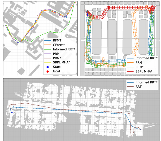
Fig. 1. Selection of environments provided by Bench-MR: City grid from the Moving AI path-finding benchmark [2] (top left), polygon-based warehouse environment (top right), and thresholded occupancy grid from the Freiburg SLAM dataset [3] (bottom).
