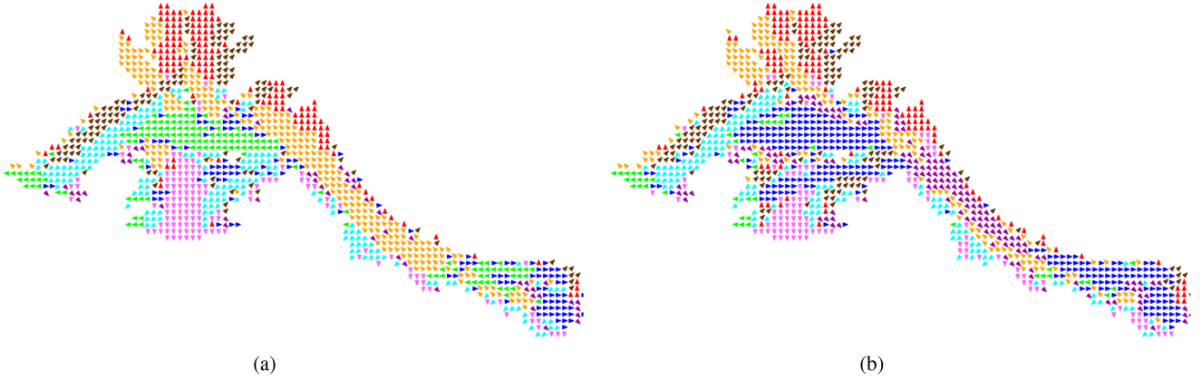
Fig. 2. STeF-Map model predictions for all cells in the ATC dataset at two different points in time in a day: 11:00 and 18:00. The arrow shown in each cell corresponds to the discretized orientation with the highest predicted probability of human motion at that point in time.
