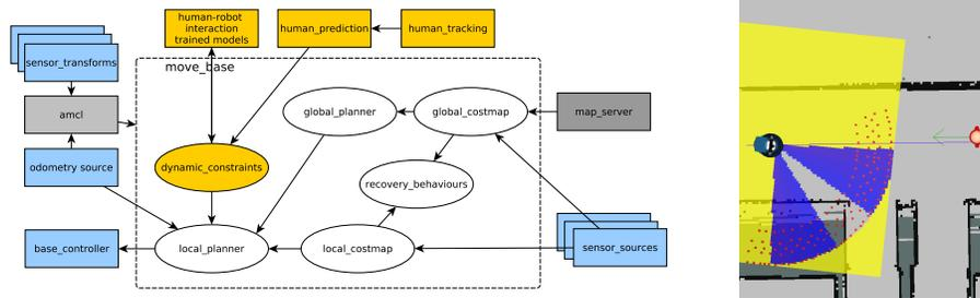
(a) Classical navigation architecture with proposed additional modules (yellow). (b) QTC-generated constraints for DWA.
