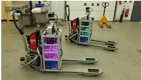
**Fig. 1.** The ILIAD robot, a Linde CitiTruck modified for autonomous operation
